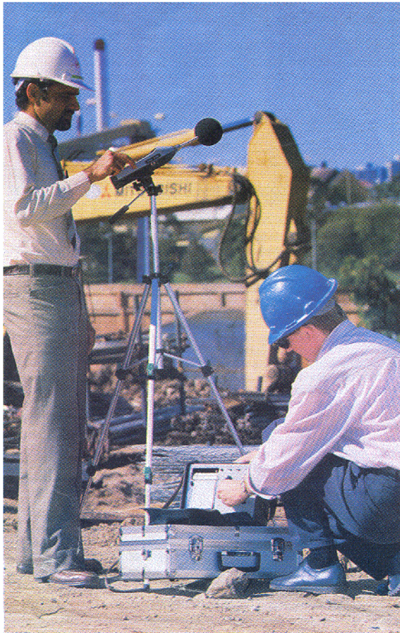
Department officers using sensitive recording equipment near a building site to obtain tapes to be used for laboratory analysis of the area's noise levels.
