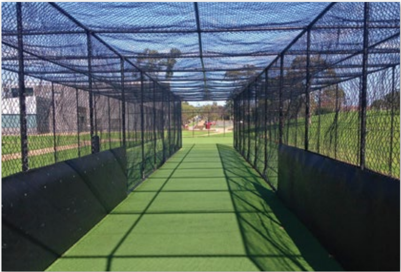
The adjacent image provides an example of a fully enclosed and roofed training net facility with ball control measures in place to prevent balls exiting the practice area into neighbouring parkland.
