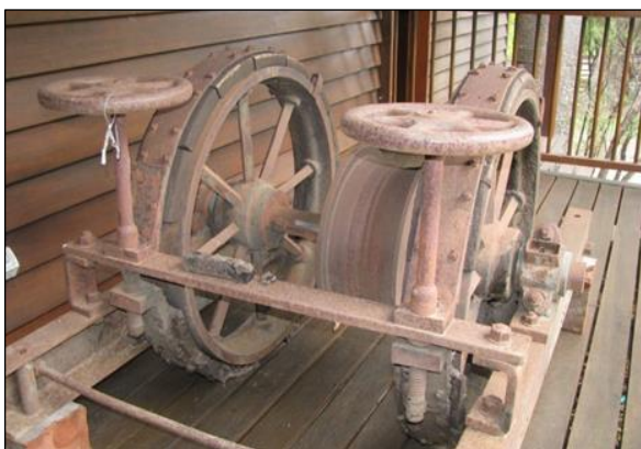
Braking gear used in a balanced incline on display at Woodworks Museum, Gympie.
