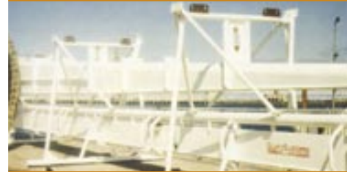
Sand Shifter system prior to burial (SlurrySystems)
