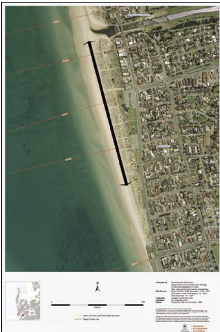
Figure 6.3 Expected residual dune width near the Torrens Outlet as a result of the five-year sand recycling program (2004–05 to 2008–09). The black line indicates the length of the beach from which sand may be removed during the five-year program. The yellow line indicates the extent of the dunes that may be progressively eroded by subsequent storms.
