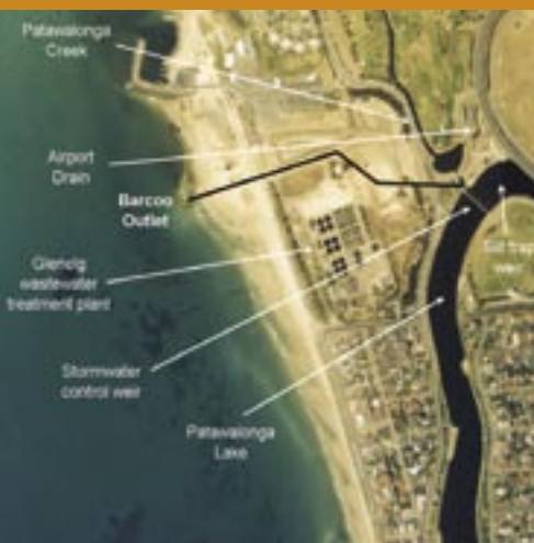
The location of the Barcoo Outlet – the buried pipeline is marked by the black line
