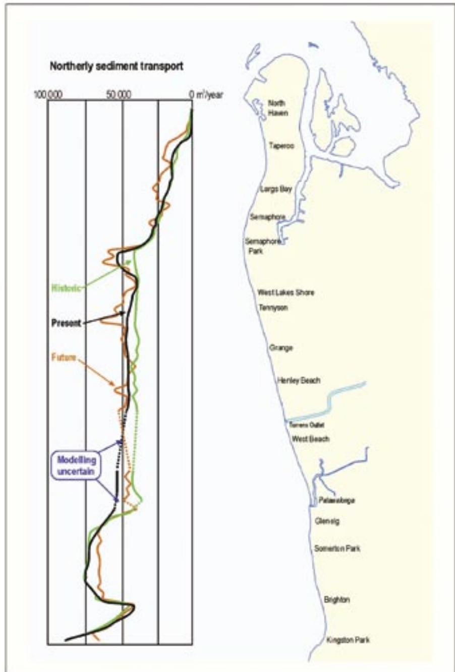
Figure 5.11 Sediment transport rates for 100 years ago, present conditions and plus 50 years
