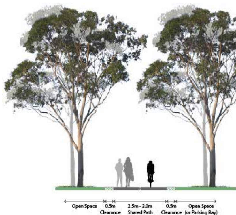
Figure 17 - Typical Shared Path cross section
